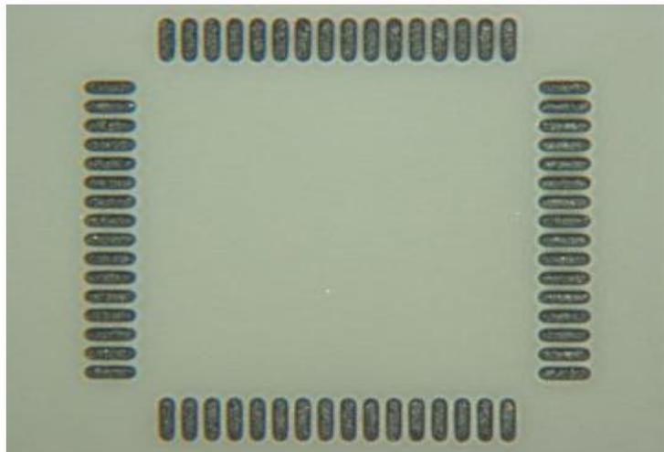
150um Thick Solder Paste Applied to the Ceramic Coupon
