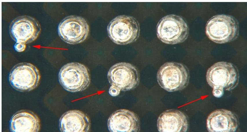
**Flipped PBGA Where Applied Solder Did Not Completely Wet the Spheres**
