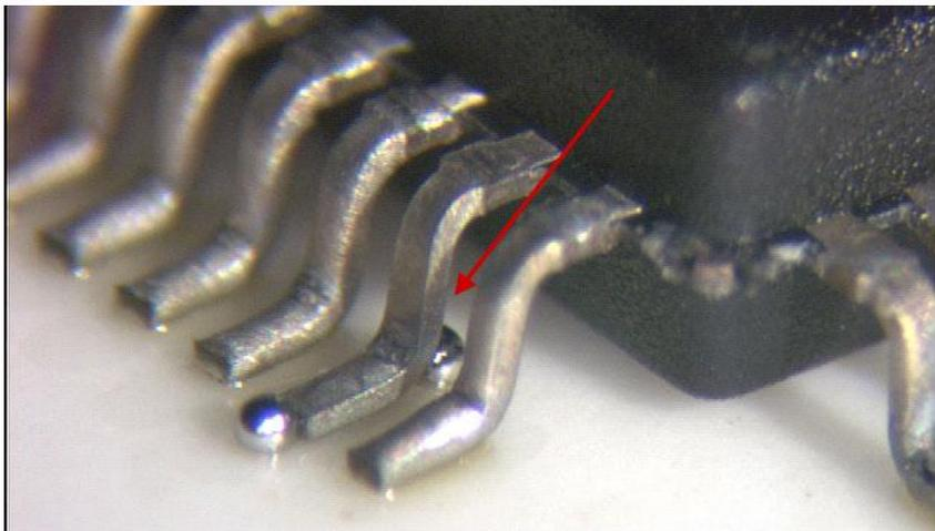
**Solder Balling Indicating Non-Wetting at the Foot on a QFP**
