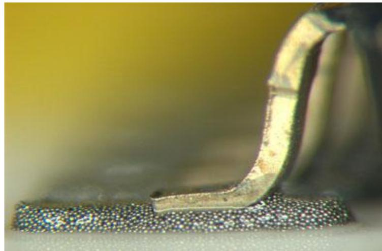
QFP Lead in Paste, Prior to Reflow
